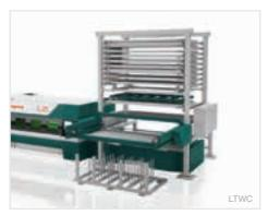
The L5 can be fed manually or automatically using the ADB and ADL connections whereby sheets are taken from one or more packs to feed the machine in masked time.
