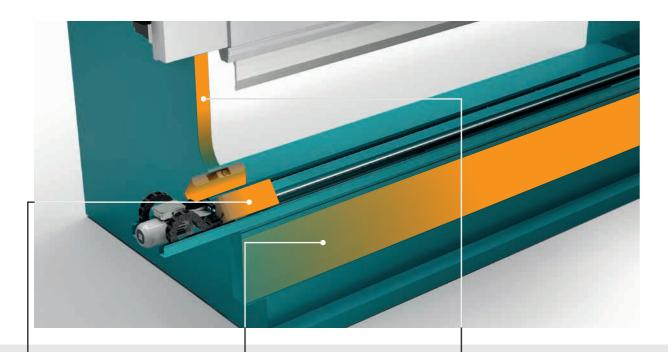
AMS - Angle Measurement System: angle measuring laser for the compensation of the sheet's spring-back. It also allows measurements to be saved and active monitoring for enhanced productivity. S-CROWNING - Salvagnini crowning: fully adaptive mechanical crowning system. It ensures consistent bending angles along the full bending length, even as parameters vary, without operator intervention.
