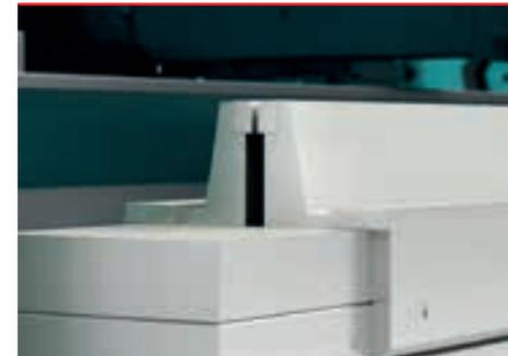
The **MVM** option, the **variable opening die which is an alternative to ATA.L**, automatically adapts the opening of the V on the basis of the program and allows materials with different thicknesses and/or bending radii to be bent. It does not require manual die set-up, increasing the productivity and flexibility of the press brake.
